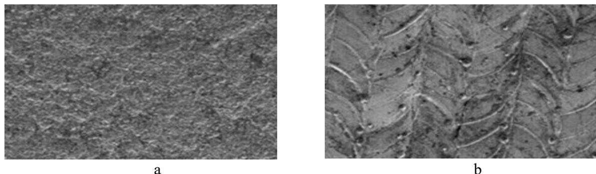
Figure 1. Surface SEM images of coatings obtained by plasma spraying (a) and laser melting (b)
