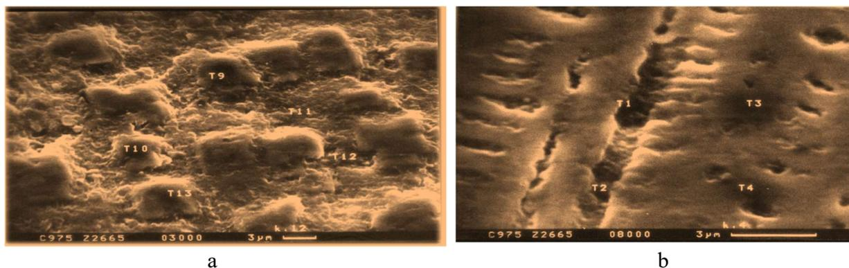
Figure 4. Structures of the formed coatings from samoflux based on iron ПР-Х4Г2Р4С2Ф alloyed with boron carbide after reflow by a continuous laser: a - laser movement speed -  $5 \cdot 10^{-3}$  m/s; b -  $0.83 \cdot 10^{-3}$  m/s.
