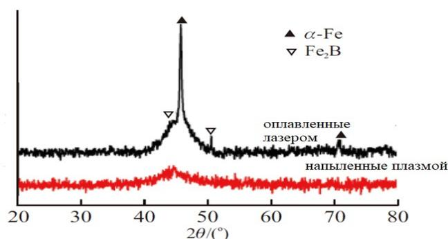
Figure 3. X-ray patterns of sprayed and laser-melted coatings
